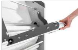
Swing-up feed table for quick set-up
